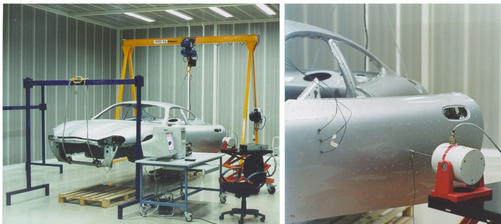
Figure 5.1: Experimental modal analysis of an automotive (Jaguar) body in white, typically done to reduce vehicle noise and vibration harshness a .
